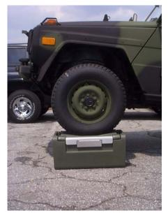
An example of the strength of our containers is clearly shown during a test and demonstration at Marine Corps Base, Camp Lejeune, North Carolina. The container is supporting the weight of one corner of the new Marine Corps Diesel IFRAM vehicle. Our containers are built tough to withstand the rigors of a battlefield while maintaining a streamline design.
